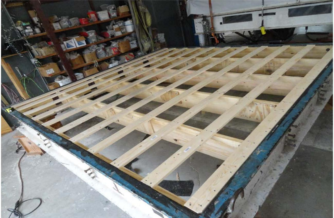
**TEST ASSEMBLY G 1x4 WOOD PURLINS BEFORE TESTING**
