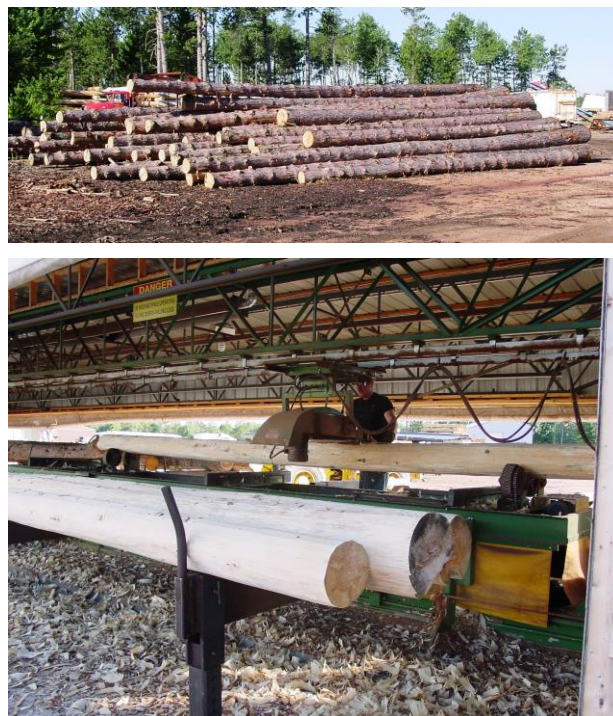
Figure 8-20. Logs prior to peeling (top) and during peeling (bottom) at Frontier Builders Inc., Land O' Lakes, WI.
